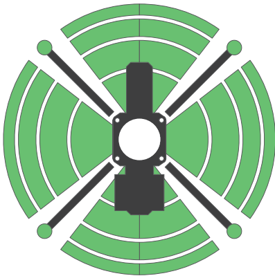
Maximum stability: Full rotation of the outriggers. Full extensions of the outriggers.
